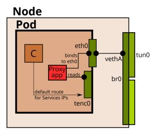
Figure 2: Overview of the proxy application implementation schema
