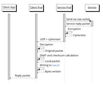
Figure 5: Traffic flow part three, Service replies to request
